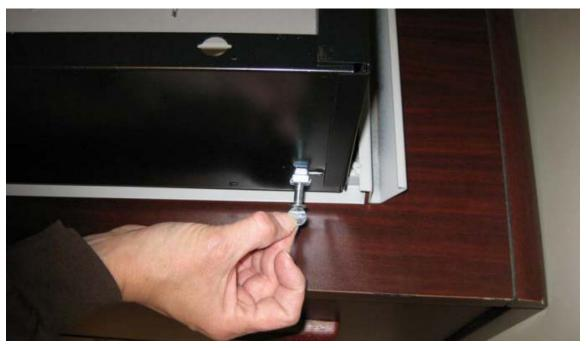
Insert from thumb screw into openings on either side of the back. Remove thumb screw and put though opening on the gondola and screw in tight to attach.
