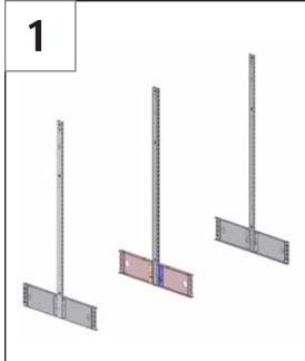
With the left upright (smooth side out) in hand, take the left hand bottom arm (smooth side out) then slide it into the upright and push down to seat the hooks.
