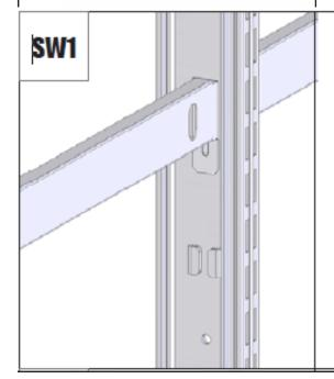
Install the slatwall tie bar by sliding it into place as pictured to the left. You may need to tap the slatwall tiebar to properly secure it.
