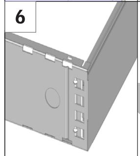
Align the kick plate tabs with the fingers of the bottom arms. Tap kick plate with your hand or a mallet to seat the tabs securely in the fingers of the bottom arm. Repeat step for opposite side.
