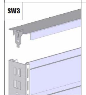
Slide the top cap over the slatwall back panels and tap with your hand to seat it. When seated the topcap should be flush across the top.
