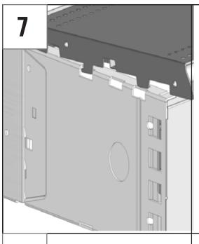
Tip the deck up slightly and slide it into the slots on the bottom arms. When installed correctly the deck should not tip forward when you push on the front of the deck. Repeat this step for opposite side.
