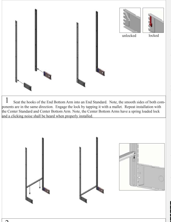
2 Install the Cross Tie by sliding it into the bottom shear form(s) of the upright. You may need to tap directly above the tab with a rubber mallet to properly seat it. See illustrations above.
