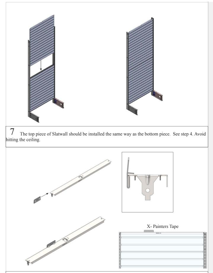
8 Determine the location of the wall stud and mark with painters tape at the top of the gondola. Slide the Top Cap Anchor Bracket as shown above. A rubber mallet may be needed to slide the bracket to the approximate location of the wall stud.
